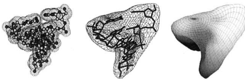
Fig. 7. Construction of principal surface with spherical topology for a distribution of points on Van-der-Waals molecular surface of a biological molecule
